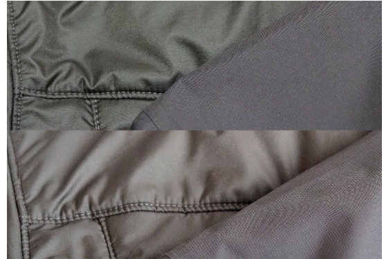
The same two fabrics, but under different light sources. The left one changes from green to brown.
